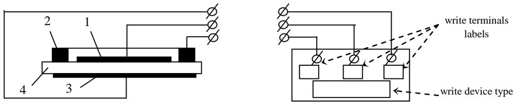
Fig. 5.3. Diagram of dielectric surface resistance measurement:
