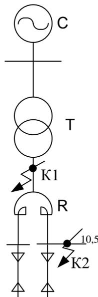
Fig. 6.1. One-line diagram of the network under study
