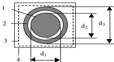
Fig. 5.1. Sketch of a sample of solid dielectric
