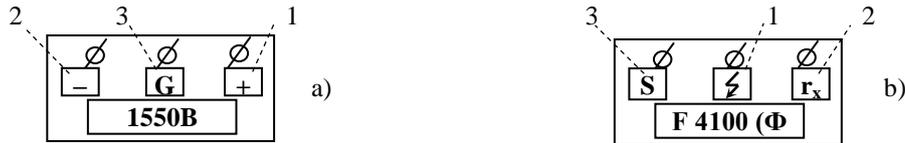
Fig. 5.4. Megger terminal designation diagrams: a – FLUKE 1550B; b – F 4100;
